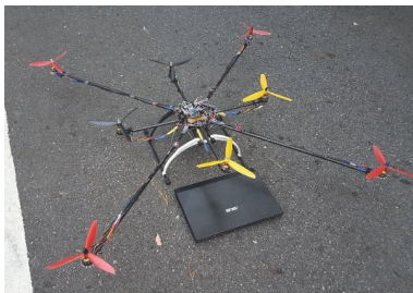
FIGURE 24: Modified octorotor to simulate QiQ stabilization algorithm.
