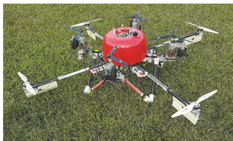
FIGURE 30: QiQ with composite fuel tank and attitude control fins.
