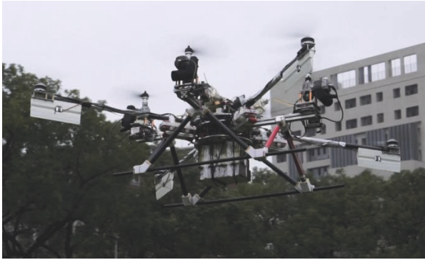
FIGURE 27: The proposed QiQ prototype in 16 kg flight test.
