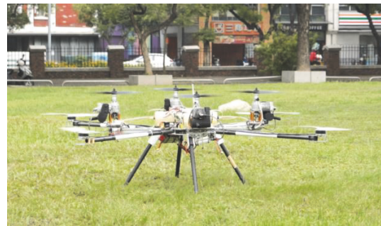
FIGURE 7: The preliminary flight test of QiQ using plastic fuel tank.
